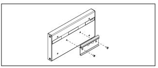
Figure 8. Compact FieldPoint DIN Rail Clip with cFP-BP-4
